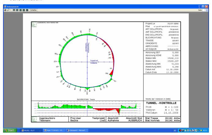
If you measure the top heading first and the side wall later - the points of side wall are automatically added to the profile in which the points of top heading already exists. you will get a whole profile without any extra work. All parameters can be changed via software.
